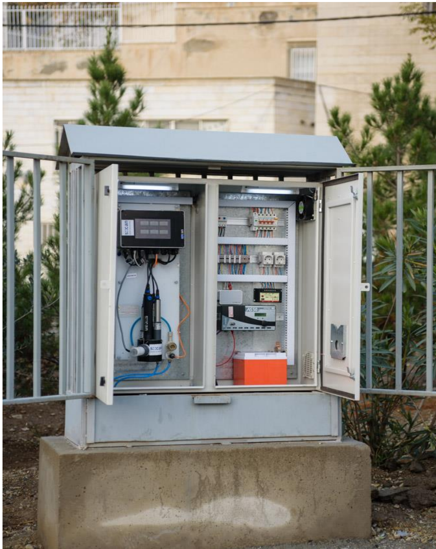
Online Water Quality monitoring station- Tehran Region 1 WWC s::can nano::station
