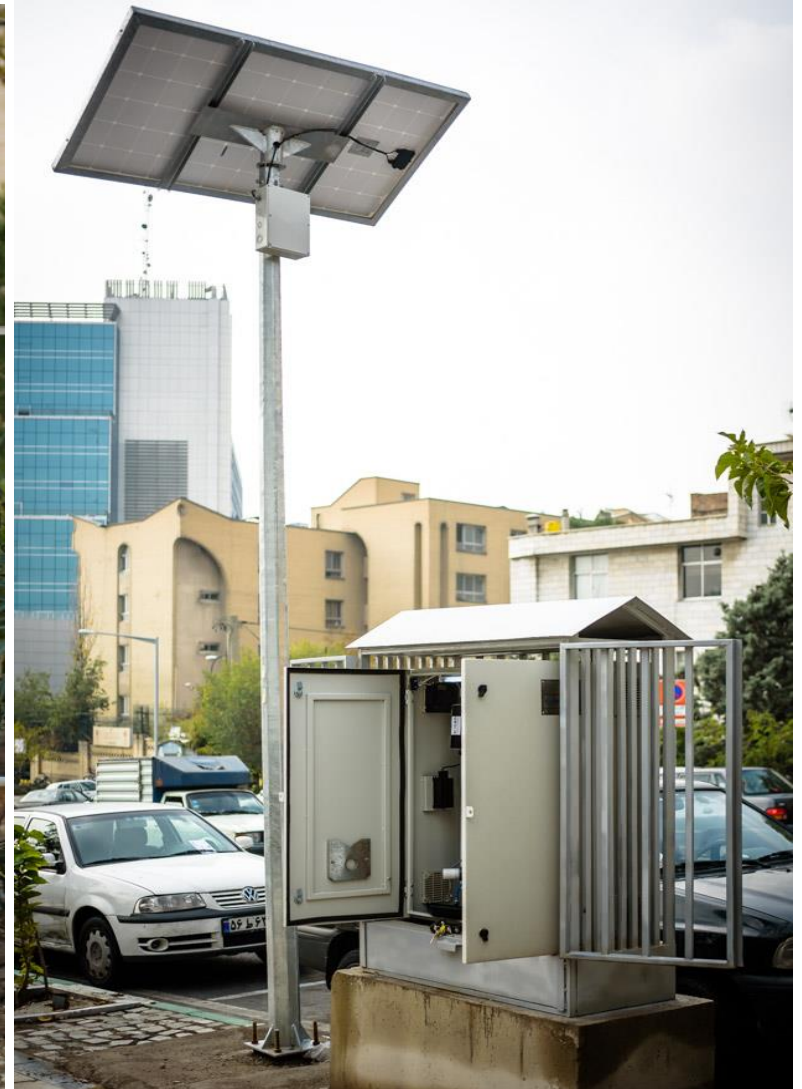
Online Water Quality monitoring station- Tehran Region 1 WWC s::can nano::station
